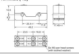
Dimensions and Operating Characteristics The solder terminal model has a suffix "-1A" in its model number and its omitted dimensions are the same as the corresponding dimensions of the pin plunger model.
